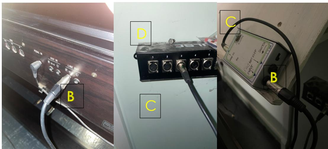
4. **Place box A** near 6 mic input box D and connect with 3pin Mic lead C to channel 3. The lectern is a good place to sit Box A.
