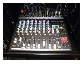
The red sliding faders on the right control the overall volume through each of the two speakers which are mounted in the hall. The grey faders control the volume by individual channel. Please do not try to adjust the other settings unless you are an experienced user.
