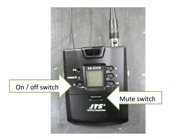
The belt pack can be used in conjunction with the attached lapel microphone. It can be turned on by pressing the bottom switch on the left. The mute switch is in the middle, below the digital display. To turn off after use, press and hold the on/off switch and wait for the "off" message in the digital display.
